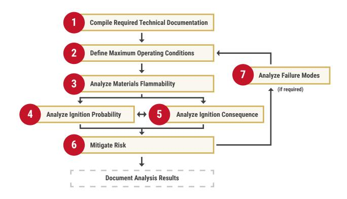
**For Step 1**, all system or component documentation is compiled. This can include piping and instrumentation diagrams (P&ID's), schematics, isometrics, component cross-sectional drawings, materials specifications, cleanliness specifications, and operating conditions.
